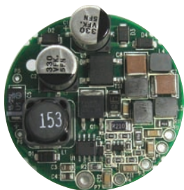
Multiple LED Driver Module
