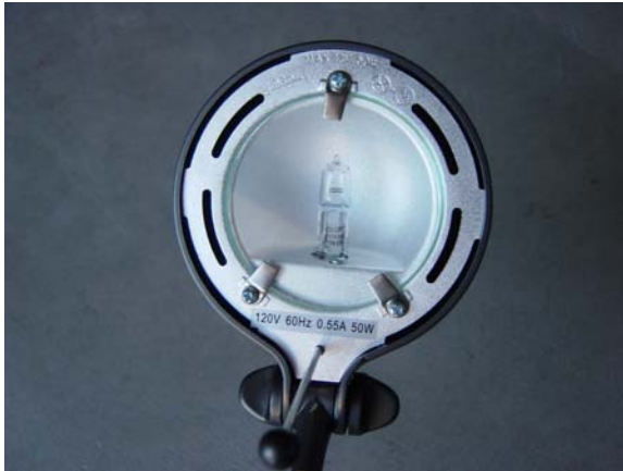
Figure 2: 50 W Bulb with protective glass removed
