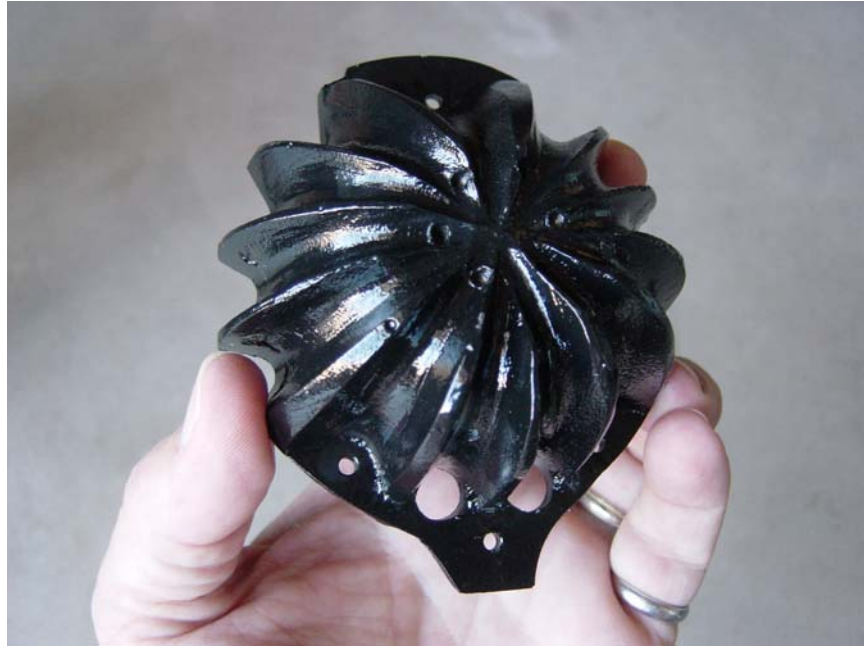
Figure 4: Custom Heatsink for Lamp Shell
