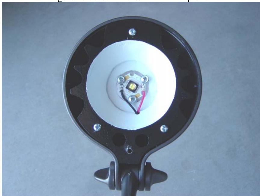
Figure 5: Cree MC-E mounted on sub-mount and connected to heatsink
